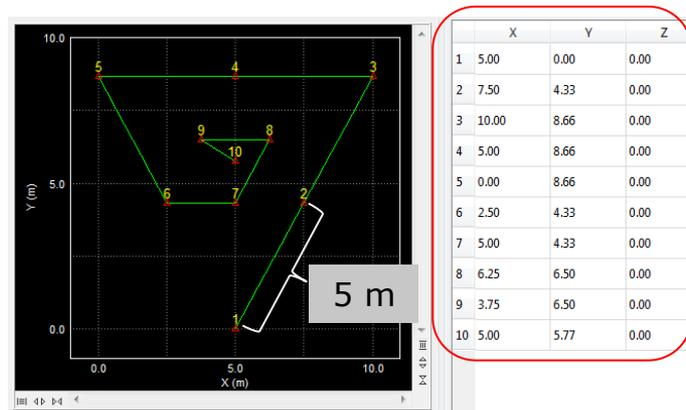
Here is a template for a 5-meter spacing cable to set up the outer side length of 10 m.
